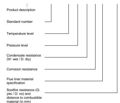
Properties of a multi-wall metal chimney system
